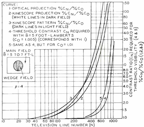
Fig. 7—Object contrast and ratio required for threshold vision.
