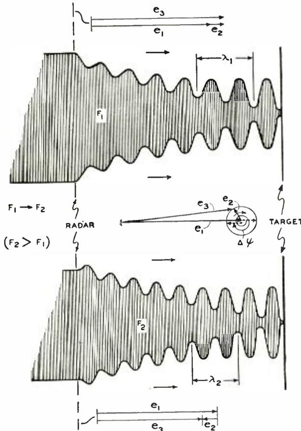
Fig. 2—Effect of frequency change on standing-wave pattern and signal-vector phase.
