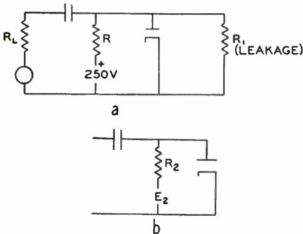
Fig. 10—The effect of leakage.
