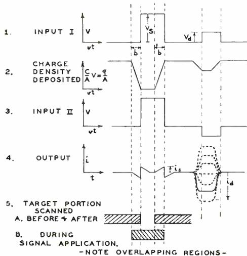
Fig. 12—Target behavior. In lines 1 to 3 the abscissa is the position ( $vt$ ) of the beam spot along the scan line on the target. Line 4 is the output signal during scan II. The dotted lines indicate schematically the variable signal output for different variations in amplitude between scans. In line 5 is shown the actual target area scanned, with that area scanned during the signal removed to the side for clarity.
