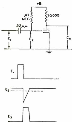
Fig. 16—Non-linear differentiator for delaying a pulse.
