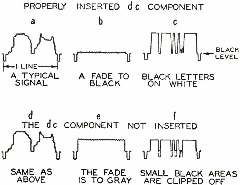
Fig. 2—Insertion of dc component.
