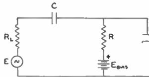
Fig. 9—Positive bias circuit.
