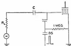
Fig. 19—The single keyed diode.
