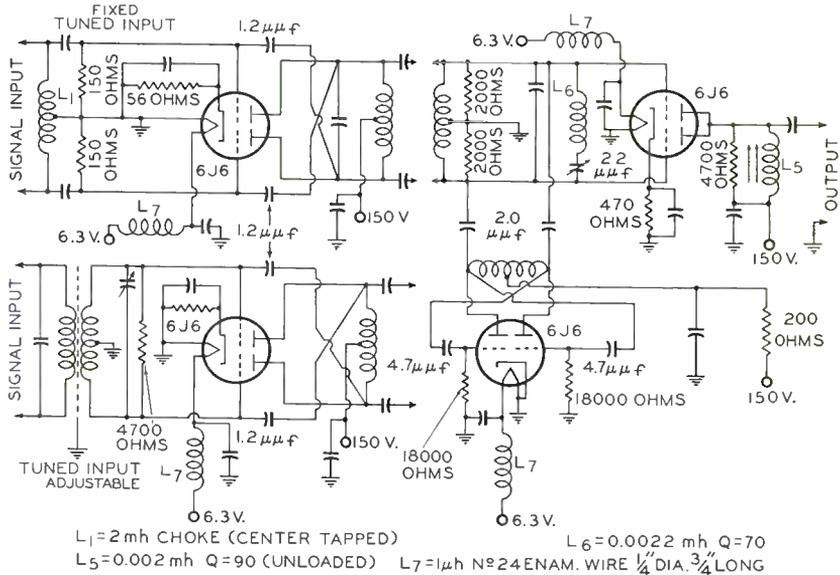
Fig. 2—Push-pull radio-frequency amplifier, oscillator, and balanced-input mixer.
