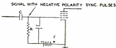
Fig. 7—Circuit in which gas current may cancel diode current.
