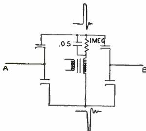
Fig. 18—The four diode clamp—used mainly for measurements.
