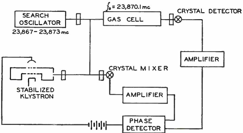
Fig. 3—Block diagram of stabilization system.
