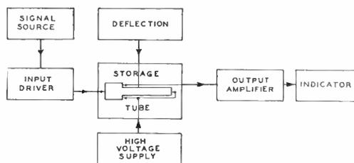
Fig. 1—Block diagram of storage tube cancellation circuits.
