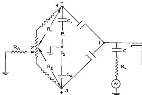
Fig. 15—Bias from double diode clamp.
