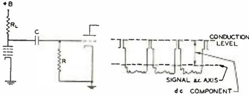
Fig. 3—The simple dc restoration circuit.
