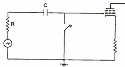
Fig. 12—The idealized clamp circuit.
