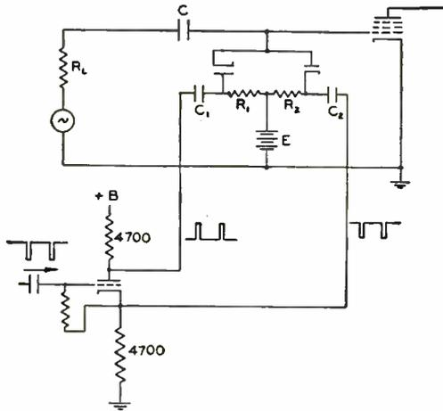
Fig. 13—The double diode clamp circuit.
