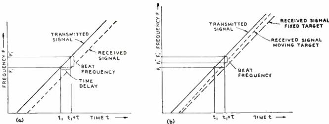
Fig. 1—Variation of transmitted and received frequencies with time.
