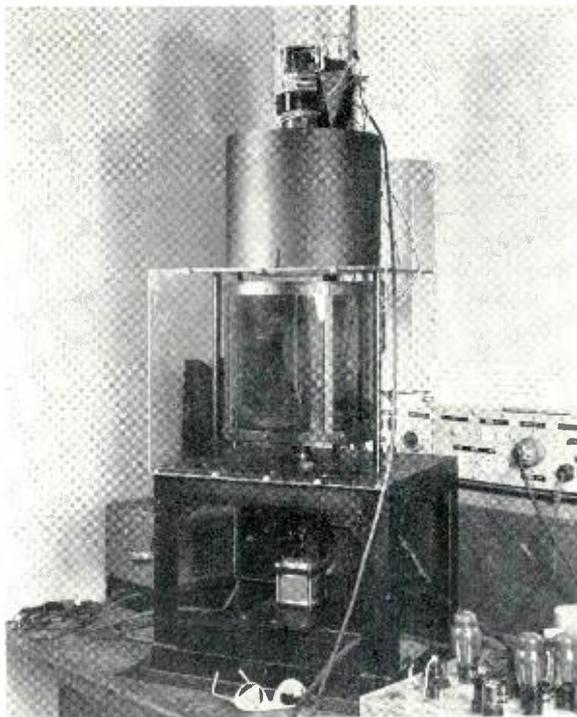
Fig. 9—Viewing device for alternate-fan-beam stereoscopic radar system.
