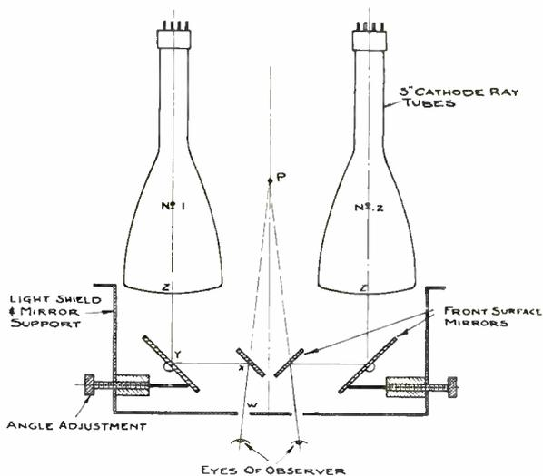
Fig. 1—Arrangement of the stereo-oscilloscope.
