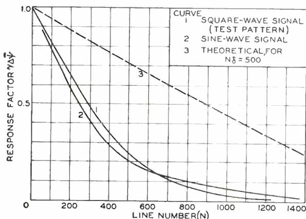
Fig. 13—Equivalent square-wave aperture response of "1000-line" kinescope.
