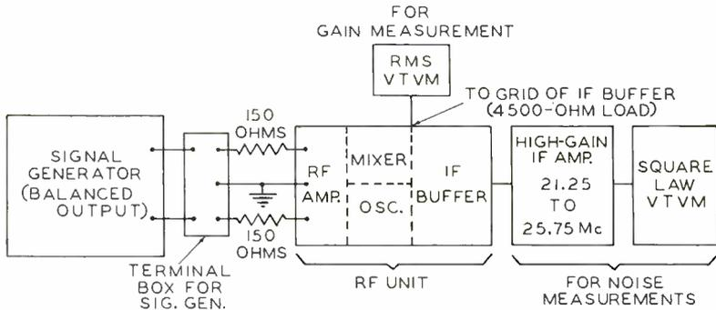
Fig. 1—Block diagram of test set-up.
