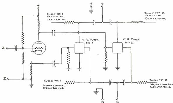
Fig. 5—Circuit for three-dimensional scan.
