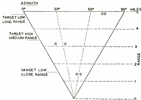
Fig. 10—Scanning pattern for alternate-fan-beam stereoscopic radar system.
