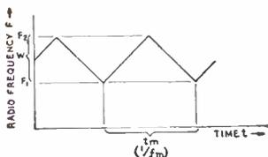
Fig. 4—Characteristics of triangular modulation.
