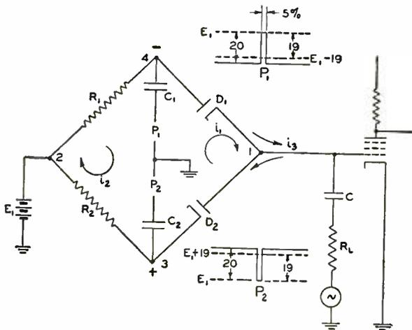
Fig. 14—Double diode clamp equivalent.
