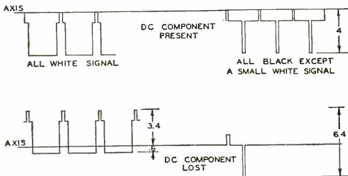
Fig. 20—Peak to peak signal with and without dc.
