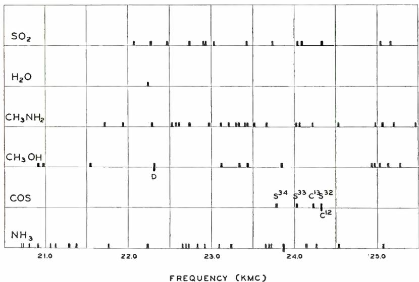
Fig. 1—Absorption frequencies for six gases.
